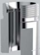
**4.1** Insert the tube end into the  $24^\circ$  taper as far as it will go and press on it. The tube must be held in as far as it will go during the entire assembly process in order to avoid faulty assembly.
