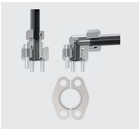
SAE flange couplings are supplied both as standard and as high-pressure designs with hole patterns in accordance with SAE J 518 or ISO 6162.
