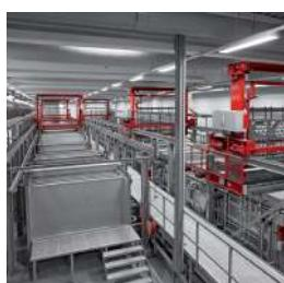
All bath parameters are continuously monitored. Chemicals are added in a fully automatic process to maintain the correct concentration.
