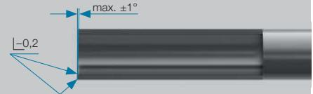
**3.3** Deburr the inner and outer edges of the tube ends slightly and clean the tubing.
