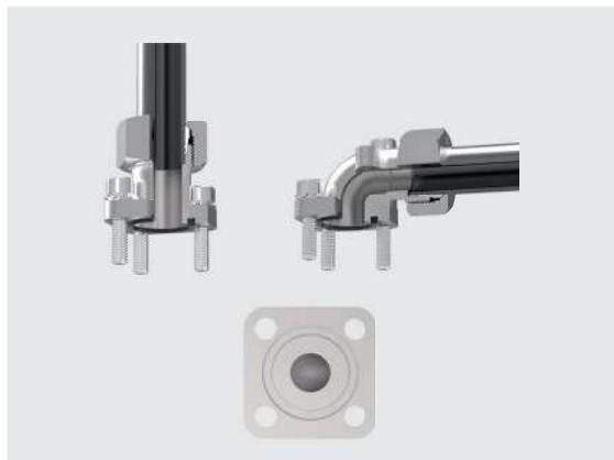
These flange couplings with a square flange connection are characterized by very compact external dimensions. Both straight and elbow versions are available. The product range covers tube outer diameters ranging from 10 mm to 35 mm. The flange connections are sealed with a circular elastic sealing ring (O-ring), and the physical connection is made using cheese-head screws. The flange connections are designed to match the connection hole patterns of leading pump manufacturers.
