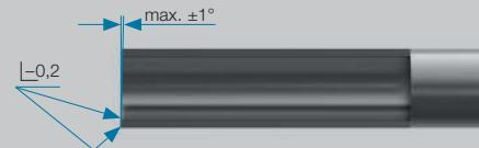
**2.3** Slightly deburr tube ends inside and outside. Clean the tube.
