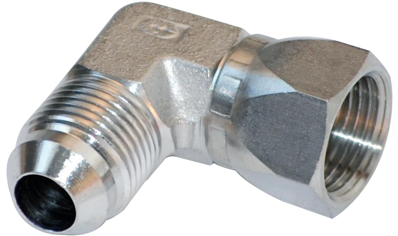
**ORDER INFORMATION** Sizes of the fittings are indicated by the dash numbers as relating to sixteenth's of an inch measured from the Outside Diameter of the tube size used. For example; 1/2" O.D. (8/16) or - 8. Male or Female pipe sizes are similar in that 1/2" pipe thread is also (8/16) or - 8.
